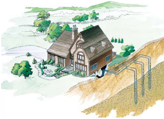
An example of a vertical loop installation
